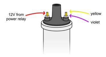
Both ignition outputs from the ECU go onto the coil negative terminal. The distributor can be left as standard but all that is now used are the rotor arm and cap; the advance mechanisms, points etc are redundant.
