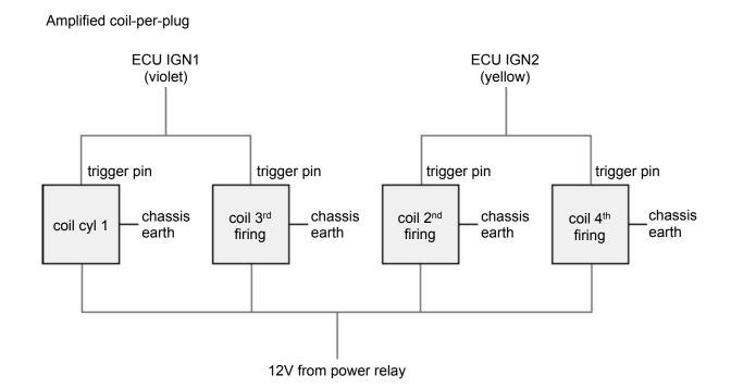
Coil-per-plug with external amps
