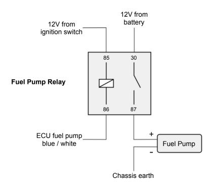
The power supply relay for the coil, can also be controlled by the fuel pump output. Though it is normal for this to be controlled just by the ignition switch.
