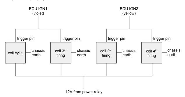
Coil-per-plug with external amps
