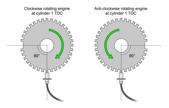
If machining a trigger pattern into the front pulley then it is usually easiest to machine all of the teeth in, mount the front pulley, and then remove the tooth pointing at the sensor at 90° BTDC.
