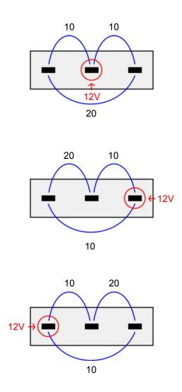
Some valves have the diodes inbuilt and will have a diode diagram on them. If so, the polarity of the wiring must be as shown below.
