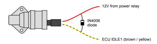
The diode in the wiring is required. The polarity of the wiring onto the valve is not important, but the polarity of the diode with respect to the wires is. The marked blocking end must face the 12V wire.
