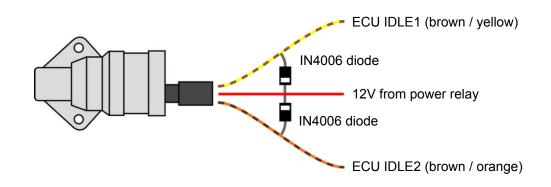
The diodes in the wiring are required. The marked blocking end must face the 12V wire.
