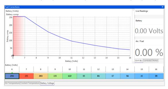
The battery voltage compensation data can usually be supplied by the injector manufacturers. For example, the Weber IW 058 injector data is for 3bar fuel pressure,
