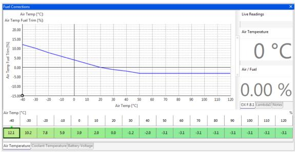
If you wish to change the fuelling with air inlet temperature, then the **Air Temp Fuel Trim table** allows the user to make a percentage change in fuel based on AIT.
