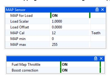
Ensure **MAP** for **Load** is **ON** and the MAP sensor is scaled as described in the sensor setup section of this manual. Set **Advanced | Boost Correction** all options **ON**.
