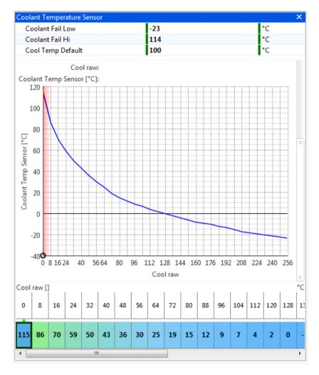
The coolant temperature sensor used by the Omex ECU is a resistive sensor. The raw output of this sensor is calibrated in the ECU to give the information in a more usable form, °C. Sensors are calibrated in the **Coolant Temp Sensor table**. The values for many sensors are known but you may
