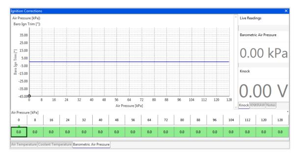
The fuel and ignition can be trimmed to allow for changes in barometric pressure as sensed by a 1bar pressure sensor. The ignition trim is defined in the **Baro Ign Trim table**. The fuel trim values are a known mathematical equation so are inbuilt and are non-adjustable.
