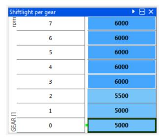
For this control a road speed sensor must be fitted and calibrated, and gear recognition must be calibrated.
