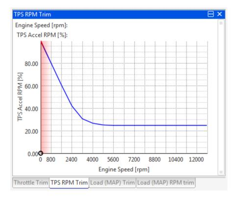
Engines usually require less acceleration fuel at high rpm, so the **TPS Accel RPM table** and **Load Accel RPM table** describe the percentage of the calculated fuel supplied at differing engine speeds.
