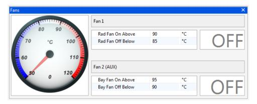
The ECU has two software outputs switchable on coolant temperature values. These would normally be used for cooling fans. The two outputs may be set to two different fans or set at different temperatures for twin speed fans.
