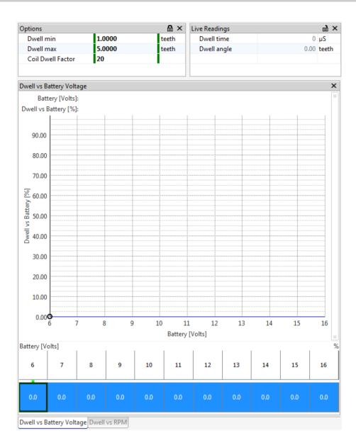
The coil dwell time is set by option **Coil Dwell Factor**. This is a unitless value typically 20 - 25 for a DIS coil pack. Charge times can be varied with respect to battery voltage and engine speed using the **Dwell vs Battery table** and **Dwell vs Speed table**. Setting these table values to 100% gives a constant dwell time.
