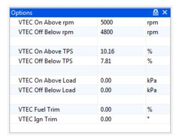
The simple on/off VTEC control is switchable on engine RPM, throttle position, and engine load with hysterisis provided by separate on and off points. In the VTEC condition there is also a fuel and ignition trim. When using TPS as load, set the Load options both to 0.
