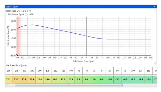
The **Idle Scatter Spark Table** shows the change in ignition timing based upon rpm away from the target engine speed. When the engine speed is higher than target negative values are required to
