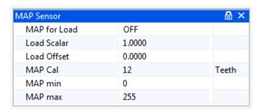
If you are using MAP for engine load sensing then set MAP for Load ON.
