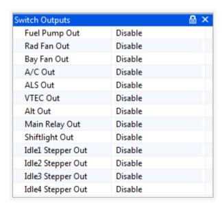
If the output needs to work in reverse (ie the output going OFF when the software function goes ON) then use the **inverted** option version.
