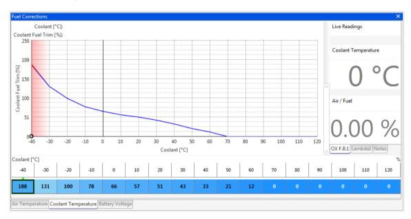
When the engine is cold, it requires an extra amount of fuel. This extra fuel is added as a percentage set in the **Coolant Fuel Trim table** of percentage increase against engine coolant temperature.
