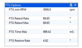
Tuning the FTG is simply adjusting the **FTG Restore Rate** for best feel. A higher value restores the power at a faster rate meaning you get back to full power quickly but you can get a shock through the drivetrain. A lower value restores the power at a slower rate so reduces shocks but too low can waste time where you could be at full power.
