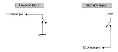
If an input is to be switched at the same time as something phsical eg a solenoid for ALS, then the physical input switch can both turnon the solenoid and give an input to the ECU.
