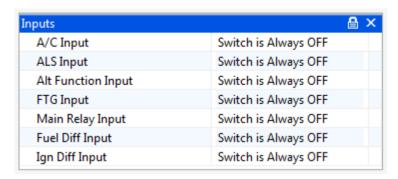
Switch input pins are selected using the drop-down options. A switch input function can have any of the input pins on the list assigned to it so long as they are not being used already by sensors. (eg. If an oxygen sensor is being used on pin OX1, a switch clearly cannot be assigned to this pin). For a function to be active always without a physical switch to turn it on (sometimes this is the case with the Alt Function) select **Switch is Always ON**.
