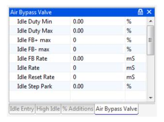
**Idle Duty Max** is the duty cycle above which the idle motor does not flow extra air. **Idle Duty Min** is the duty cycle below which the idle motor does not flow any air.
