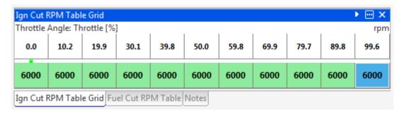
At this engine speed, the soft cut will be invoked. If the engine speed is exceeded by 50 rpm, then the hard cut is invoked. If you are not using a cam sensor so have semi-sequential fuelling, the **Fuel Cut RPM Table** should be set to an engine speed that is higher than the ignition cut rev limit.
