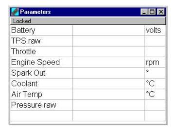
As some of the sensors have been checked during calibration, there are only a few remaining. **Battery** is the battery voltage and should read between 9 and 16 v. The coolant and air temperatures should read sensible numbers, around room temperature if the engine has not been started. **Engine Speed** will show between 100 and 250 rpm under cranking. This can be checked when the timing is calibrated.
